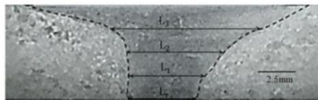
Figure 2. Weld-zone macrostructure
