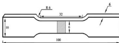
Figure 3. Workpiece dimension (mm) for testing tensile strength
